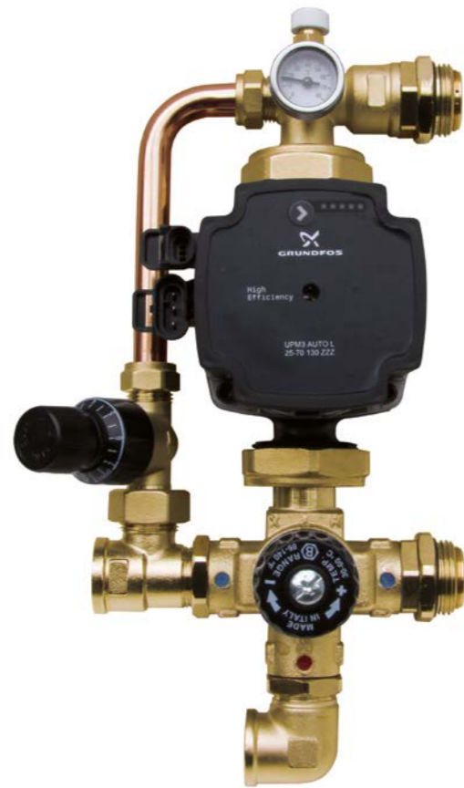
18B.1 Built-in distribution group with thermostatic mixing valve 25-50°C and differential by-pass (setting 2 - 6.5 m). The group is supplied with temperature gauge in a single bag and an integrated air vent. Fitting for manifold connection included and elbow for the primary circuit connection. (on request surface treatment)
